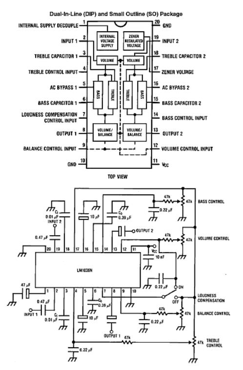
Fig. 4.2.7 The LM1036 Audio Control IC
