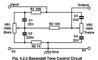
considerable attenuation (about -20dB) introduced by the passive network, and to provide true bass and treble boost. There are still many variants of the circuit in use, both as active circuits (with amplification as originally proposed), and as passive networks without an incorporated amplifier. In passive variants of the Baxandall circuit, extra stages of amplification may be used to make up for the approximately -20bB attenuation caused by the circuit.
