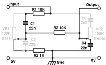
Fig. 4.2.4 The Circuit with VR1 and VR2 at Minimum
