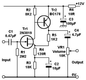
Fig. 4.3.2 High Impedance JFET Input Stage
