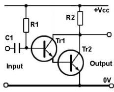
Fig. 4.3.7 The Darlington Pair with Common Emitter Output
