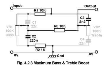
considered to be open circuit. Nor does C4 contribute to the operation of the circuit because of the high resistance of VR2, and C1 is effectively shorted out by the wiper of VR1 being at the top end of its resistance track.
