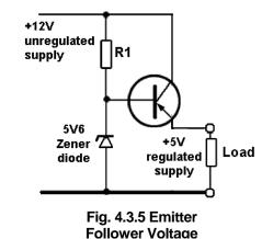
Notice in Fig.4.3.5 that the Zener diode has a voltage rating of 5V6 (meaning 5.6volts), this will maintain the base of the transistor at that voltage, and the emitter of the transistor at 0.6V below the base voltage, will be maintained at 5 volts. A small current maintaining the base voltage at 5.6V is therefore able to accurately control a much larger current flowing through the collector and emitter.
